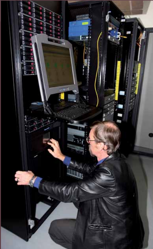
DCOSS Project Manager, Mark Denbow, configuring the tape library backup. Photograph by Kerstin Styche.
