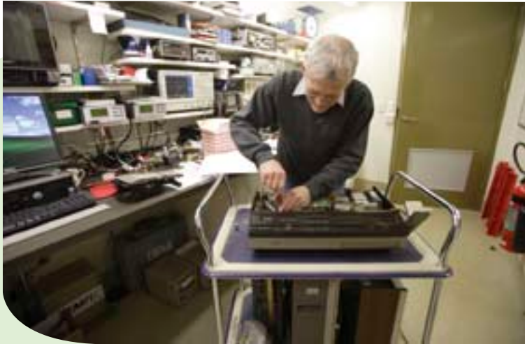
Left: Technician Doug Smith at work on the Philips N1700/45 half-inch videotape player. Right (l-r): Technicians Graham Dyson and Rob Hansen at work on the restored Sony AV3670CE video-recorder
