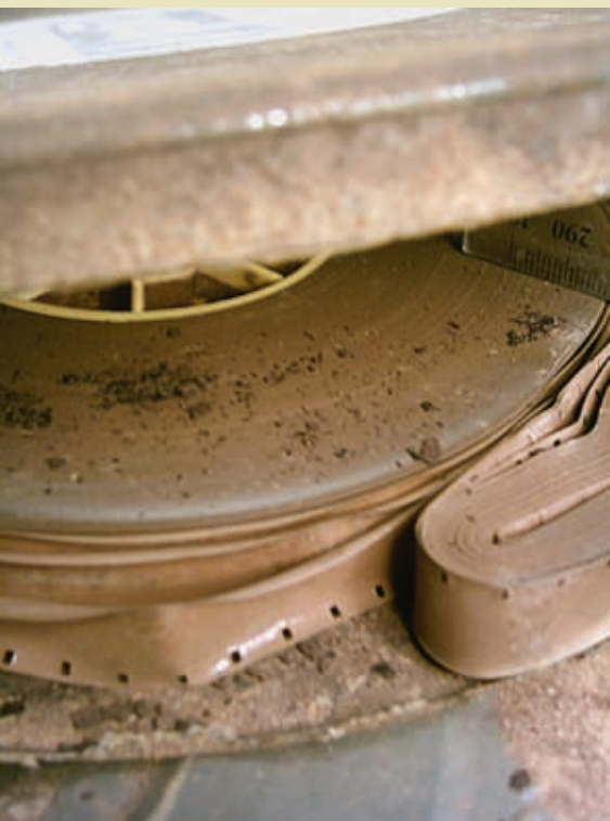
Severely degraded soundtrack to the previously unidentified Geoffrey Bardon footage. Photo courtesy of AIATSIS.
