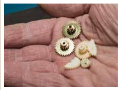
● The freshly manufactured brass gears and their nylon counterpart.
