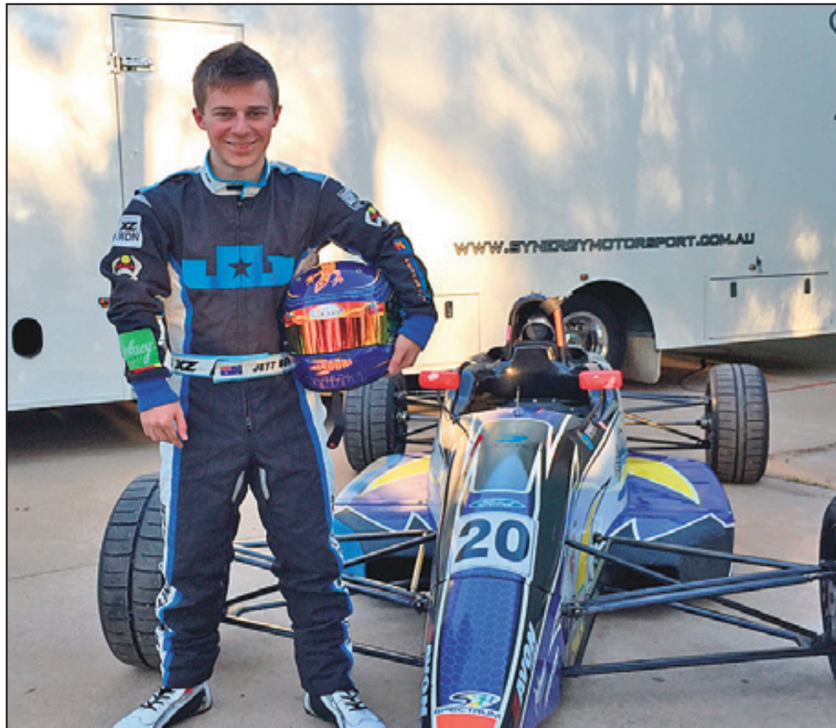
Jett Bennett stands beside a Synergy Motorsport tubular space-frame Formula Ford open-wheel car, powered by a 600cc 125hp Ford Fiesta engine.
