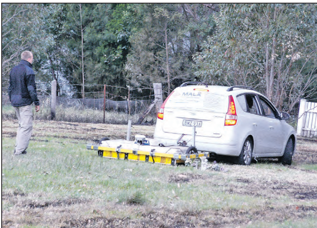
This towed GPR machine was the main one used for mapping ground disturbance in Wallaga Cemetery which will be used by geophysicists to locate past burials.
