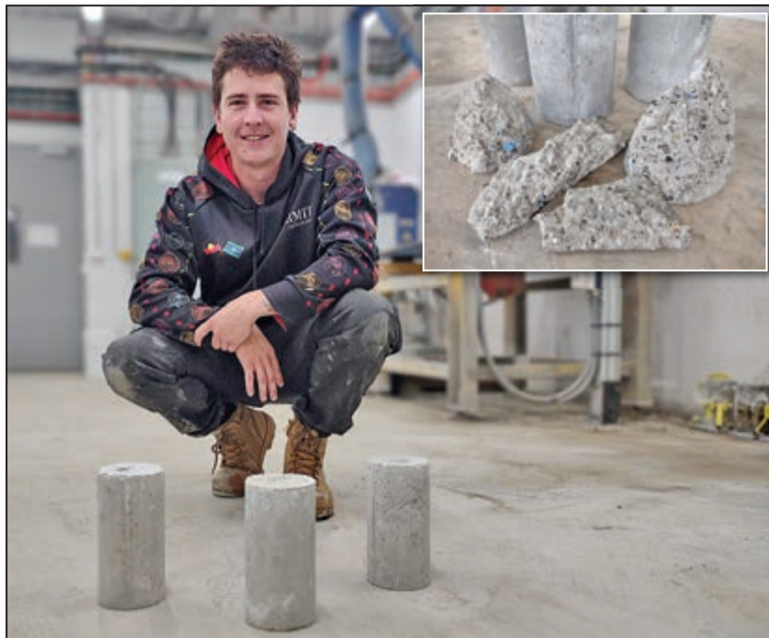
Vice-Chancellor's Indigenous pre-Doctoral Fellow at RMIT and co-researcher, Taungurung man Shannon Kilmartin-Lynch with the team's concrete that was made using PPE. Inset: RMIT University's School of Engineering team are the first to investigate recycling three key types of PPE into concrete. Pictures: RMIT University
