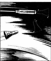
the unmanned target vehicle. The astronauts are aided by their own radar and information from ground stations in making the correct maneuvers required to intercept Agena. When the distance between the two craft is reduced to 67 kilometers, the astronauts fire a powerful rocket burst which boosts them into a position slightly ahead of and facing Agena. Both craft are now in the same orbit and traveling at the same speed—about 32,000 kilometers per hour. However, there is no sensation of speed—
